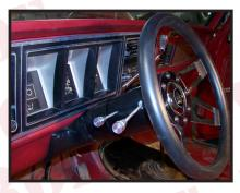
the splines. Place wheel nut on top of wheel and torque wheel nut to 35lbs.
