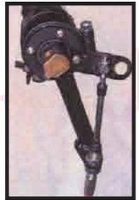
7. Reinstall the shift lever as close to the swivel as possible. Now you could turn the bracket or loosen the large nut and adjust so that the swivel goes into the 5/16" hole that you drilled in the shift arm. Insert the cotter pin in the swivel, tighten the large nut and bolt on the bracket. Do not tighten so much that it squeezes the delrin bushing in the bottom of the column. This could make it hard to shift. Remember, the cable has to be pushed down completely.
