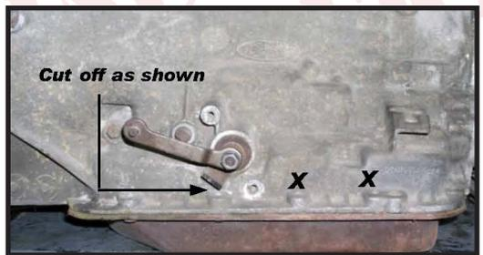
Also remove the nut and washer from the kick down lever and then remove the kick down lever itself.
