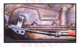
position. Now you are going to put the swivel onto the threaded end of the cable and turn it until it lines up with the forward hole of the shift lever. Install the cotter pin. If it needs more travel, loosen the large nuts and washers and move the cable forward or backward to gain more travel. Then retighten the large nuts and washers. Install the small nut and tighten.
