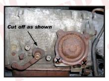
10. Make sure that the transmission is in Park. Install the transmission shift lever using the nut and bolt supplied. Now install the kick down lever with the original nut and washer as shown above. Install the cable bracket and the two bolts as shown above.
