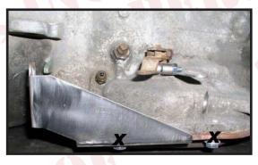
10. Spacers need to be placed between the bracket and the transmission pan with the two bolts that were marked with X's holding it all together in the holes of the bracket as shown.
