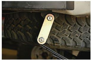
the truck. Use a small dab of grease on the threads of all the greasable suspension bolts before installing the crimp nuts.
