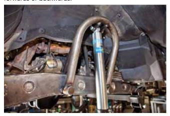
**STEP 97**Install shock hoop support tubes.
