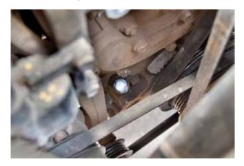
**STEP 26**Locate the small freeze plug approximately 2" behind motor mount.
