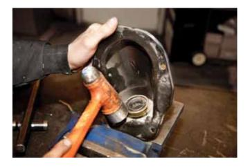
**STEP 110**Install the seal housing into the firewall.
