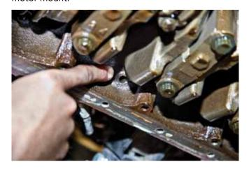
**STEP 28**Install the new dipstick tube into the block using ultra grey at the mating surface.
