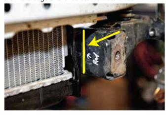
**STEP 5**Unbolt and remove all IFS components.
