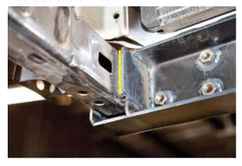
**STEP 15 A**Install spring hanger gussets in location shown
