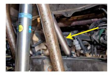
**STEP 99**Weld previously cut brake line tab to frame as shown.
