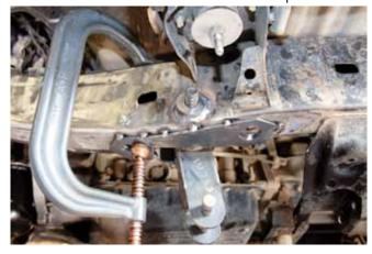
**STEP 75** Finish welding the bottom support plate.
