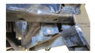
**STEP 16**Cut the brake line tab off as shown for future use.
