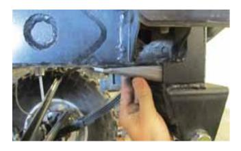
**STEP 15 C**Completely weld part as shown. Repeat on opposite side.
