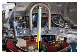
**STEP 100**Tack weld the body mount gussets into place.
