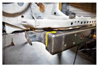
**STEP 15 B**Remove paint, and prep for welding
