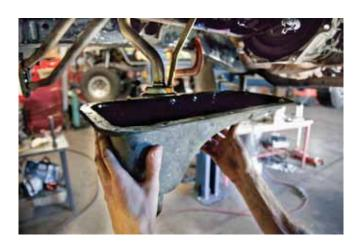
**STEP 40**Using a razor, clean the oil pan mating surface on the block.
