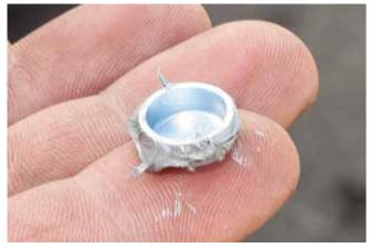
**STEP 25**Lightly tap freeze plug to secure it into place.
