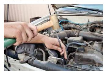
**STEP 27**Using a punch, remove the freeze plug.
