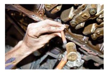
**STEP 24**Place freeze plug in stock dipstick hole.
