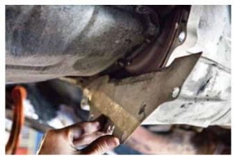
**STEP 39**Remove the stock strainer and replace it with the new one.
