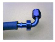
4. Put the swivel end at center hex in a vise. We recommend a vise jaw protector such as JEGS #555-80548 to protect the hose end against scratching. Using a twisting motion, make the bottom of the hex even with the hose edge.
