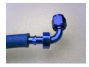
4. Put the swivel end at center hex in a vise. We recommend a vise jaw protector such as JEGS #555-80548 to protect the hose end against scratching. Using a twisting motion, make the bottom of the hex even with the hose edge.
