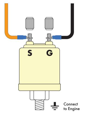
Automotive circuit connectors are the preferred method of connection. The wires can be soldered.
