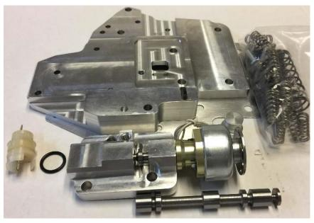
Includes: Solenoid Small parts kit (Direct drum springs, bolts and check ball)
