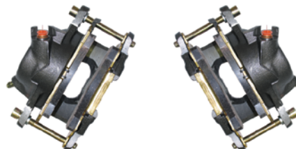
Part #: 4039 (right) 4040 (left) Calipers Uses D52 pads
