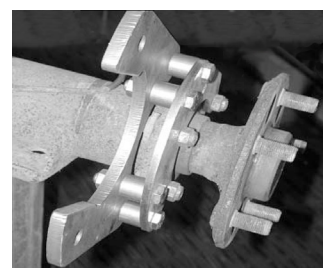
Installation of caliper bracket.
