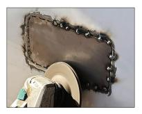
15. Once the fill panel is fully welded in place, use an angle grinder to grind the welds flush. Additional welding may be necessary.
