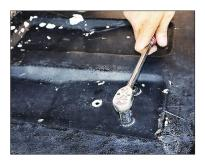
Open the tailgate and remove the (3) bolts from back that hold handle in place.
