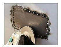
15. Once the fill panel is fully welded in place, use an angle grinder to grind the welds flush. Additional welding may be necessary.
