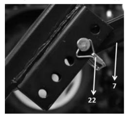
• Attach the T-shape connector with the assembled base and crane to get the tool ready to operate.
