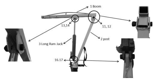
7. Assemble the hook with chain (8) to the end of the boom (1).
