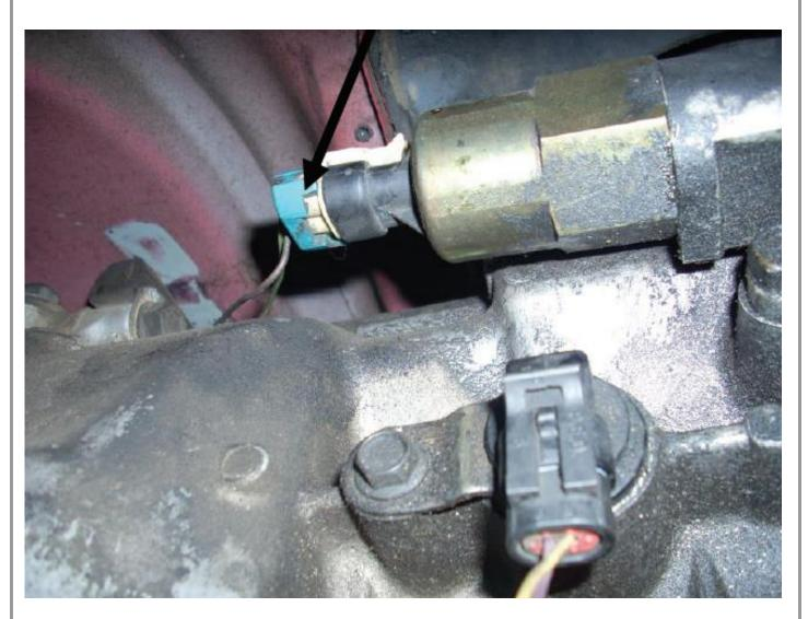
**Using an Ohm Meter** – Check Resistance Between "Negative Ground" (Chassis/Frame) and each of the 2 existing vehicle VSS wires in the vehicle harness to determine which wire is the "VSS Reference" wire and which is the "VSS Signal" wire. If you have no existing vehicle wiring, skip down to #4 below.
