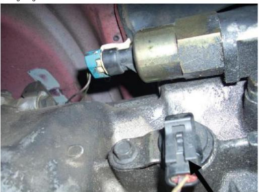
You Will Need To Disconnect and Tap Into VSS Signal Harness Wiring
