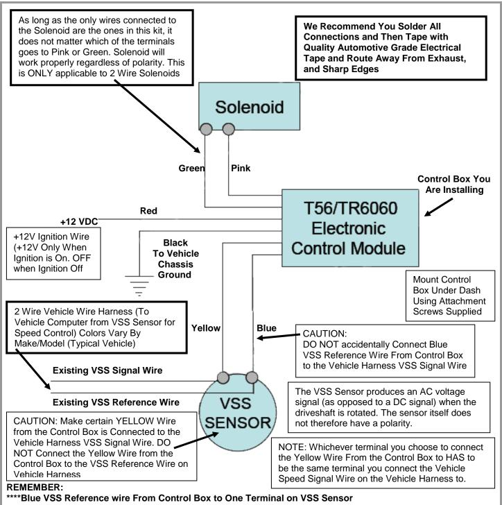
\*\*\*\*Yellow VSS Signal Wire from Control Box to One Terminal On VSS Sensor and To VSS Signal Wire on Vehicle Harness
