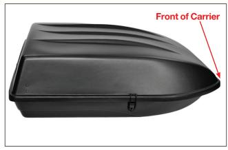
Close the cargo carrier. Pull up on the lid at the front of the carrier to be sure the hinge tabs are engaged.
