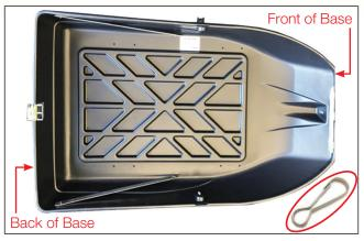
Place the base on the ground. Remove all 4 clips (#6) located on cargo carrier. You will reinstall them on the cargo carrier in later steps.
