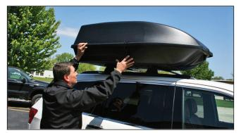
Carefully place the assembled cargo carrier on the top of roof rack cross rails and center on vehicle. Check for clearance of rear hatch and antennas.
