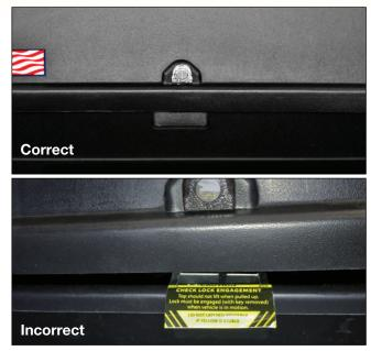
Be sure cargo carrier is fully closed. When this occurs, the yellow warning label will no longer be visible.
