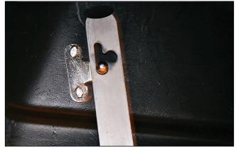
Raise the two uprights and place into the locked position on the bracket as shown.
