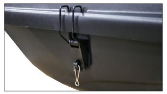
Close the carrier. Be sure that both side alignment brackets are not visible. Close the bale latches on each side, and insert clip hooks to secure.
