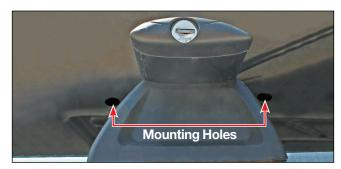
Be sure to align the mounting holes in the box bottom on each side of the cross rails.
