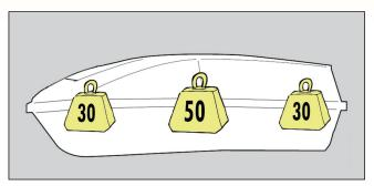
Load cargo carrier paying careful attention to distribute the weight evenly and not exceed the maximum allowed weight of the box or cross rails.
