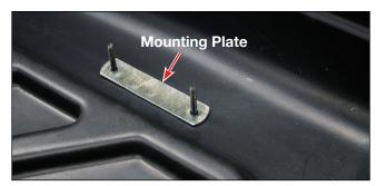
Then slide the mounting plate (#4) over the threaded posts inside the cargo carrier.
