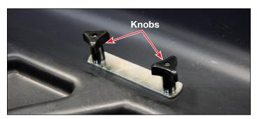
Thread 2 knobs (#3) evenly and loosely – do not tighten all the way at this point. Repeat steps until all 4 mounting brackets (#5), all 4 mounting plates (#4) are in place and the 8 knobs are loosely in place. Make sure cargo carrier is centered on vehicle. Then tighten all 8 knobs evenly and securely.
