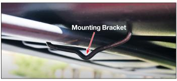
Place the mounting bracket (#5) through the predrilled holes from below the vehicle cross rails as shown above.
