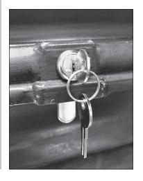
On top shell make sure all four cams are in the unlocked position and in their slots.
