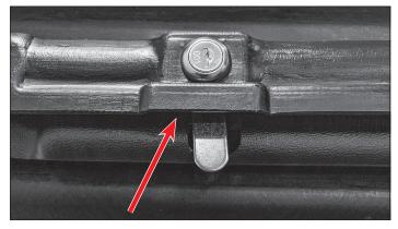
Lock cam is not in slot and not behind bottom shell.
