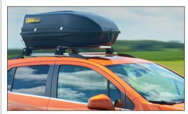
Cargo carrier should be pointed in the same direction as the front of the vehicle.
