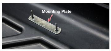
Then slide the mounting plate (#4) over the threaded posts inside the cargo carrier.
