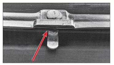
Lock cam is in slot behind the bottom shell.
