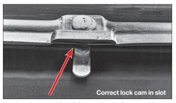
Lock only one side of the carrier before positioning it on the cross rails. Depending on which side you prefer to load the carrier. Place the opposite side locks into the locked position which will now become the locked hinge side.
