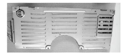
2. Remove the six(6) 7/32" screws securing the back panel.
