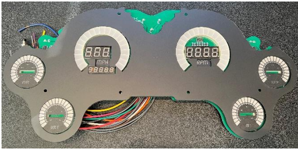
Place overlay on top of the gauges
