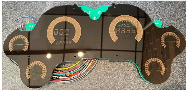
Place Acrylic over circuit board and overlay
