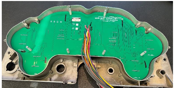
Insert circuit board assembly into housing
