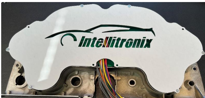
Secure the back plate to the housing using provided spacers and factory screws
