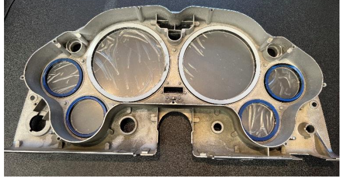
Place the 6 clear lenses and 6 spacer rings into the bezel
