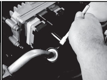
Fig # 4 tighten extender bolt
