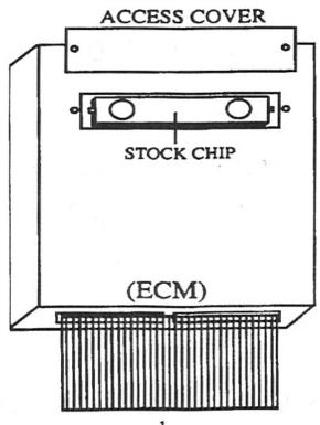
3. In some cases, it is necessary to remove the top half of the ECM to install the 6-PAK chip. To do this, remove all the external screws that hold the ECM together (most have 6 to 9 screws) and remove the top half of the ECM.
