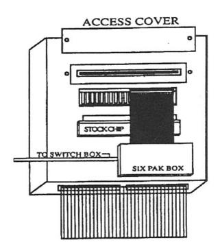
7. Replace the top of the ECM, guide the 6-PAK through the hole, put screws back in the ECM. Remove the adhesive cover and stick it to the top of the ECM.
