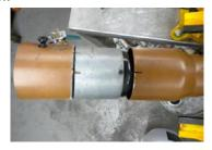
You can now install your pre-assembled steering column with electric motor. You will now need to clock the motor, mark its exact location (3 o'clock) on the column then take the column back out, drill and tap the column to the electric motor to avoid it from turning as shown in the pictures.
