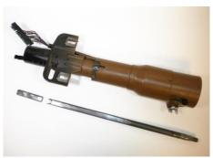
Then cut 3 % " of the steering shaft, the shaft will then slide into the %" DD on the electric motor and tighten the two set screws.
