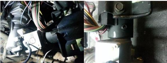
3. Once the steering column is removed, measure out 15.50-15.75" (40cm) (not including the acaridan steering wheel hub.) Start measuring from the start to the column down with a total length of 15.50-15.75" (40cm)
