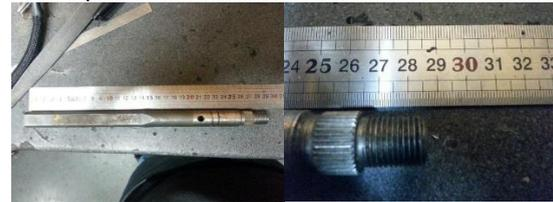
5. Attached the inner shaft into the 3/4" DD cupler on the end of the EPAS motor, that is welded onto the motor. Be sure to tighten down the 2 set screws on the cupler that is welded onto the motor, to hold the shaft in place.
