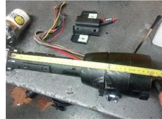
4. Measuring the inner shaft, from end to end, measure out 11.6"(29.5cm) This shafts length should be 4" overall shorter than the column. This length will be to adapt to the new EPAS cuplers and shaft.
