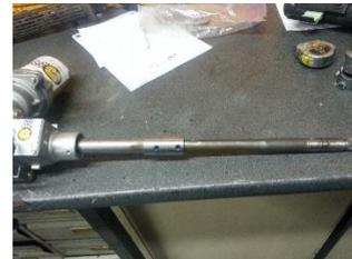
6. At this point you want to slide the steering column over the inner shaft, be sure the column fits snugly over the aluminum cupler and the column covers most of the cuplers width.
