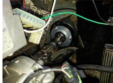
14. With the 1" DD shaft, slide into the ¾" DD, and the ujoint going to the steering box. Both ¾" DD shafts should sit inside of each other by about 2". Re adjust if needed.
