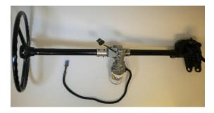
11. Install the pre-wired control module on the firewall just next to the fuse block (or elsewhere), hook up the power wire for the motor (blue connector) and the connector for the torque sensor (Delco weathepack). Then hook up the small red wire to a hot in run and the #10 red wire directly to your battery or a direct power source. You can use a 60A fuse if desired.
