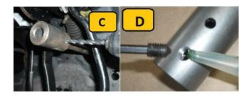
7. Never drill hole from side to side. Set screws must be flush!
