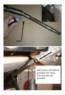
9. To see and tighten several set screws you will need to drill a 1" hole through your steering column.
