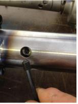
10. The aluminum color will also remain with the set screws and the coupler bolted to the back of the electric motor will also use set screws (you can weld once you have it in place and clocked).
