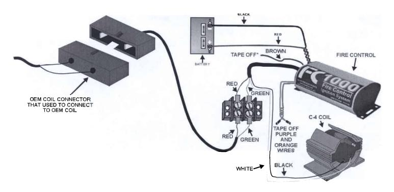
\* NOTE: If using aftermarket tachometer it may trigger correctly off the Green points connection wire in the harness. If tach bounces or fails to read, connect to Brown Tach lead off unit.
