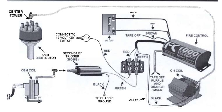
\* NOTE: When using Secondary Trigger any pre-existing stock or aftermarket tachometer should trigger off the OEM coil negative or can be hooked to the Brown wire off the unit.
