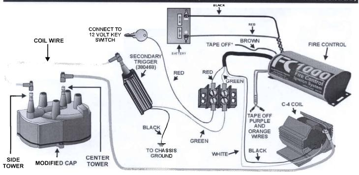
\* NOTE: When using Secondary Trigger any pre-existing stock or aftermarket tachometer should trigger off the OEM coil negative.
