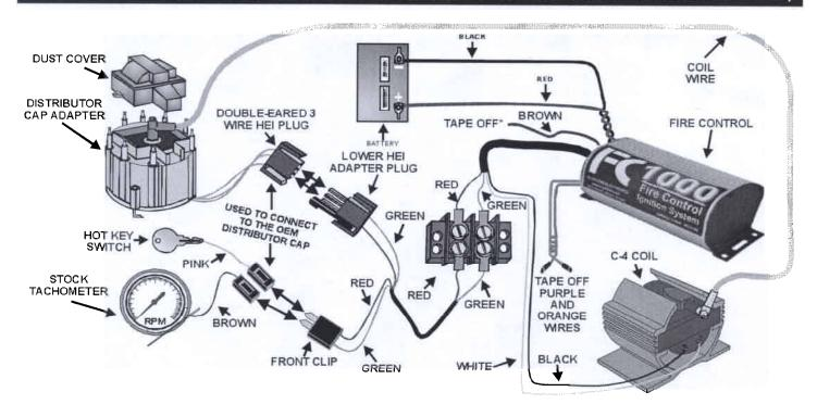
\* NOTE: If using aftermarket tachometer it may trigger correctly off the Green points connection wire in the harness. If tach bounces or fails to read, connect to Brown Tach lead off unit.
