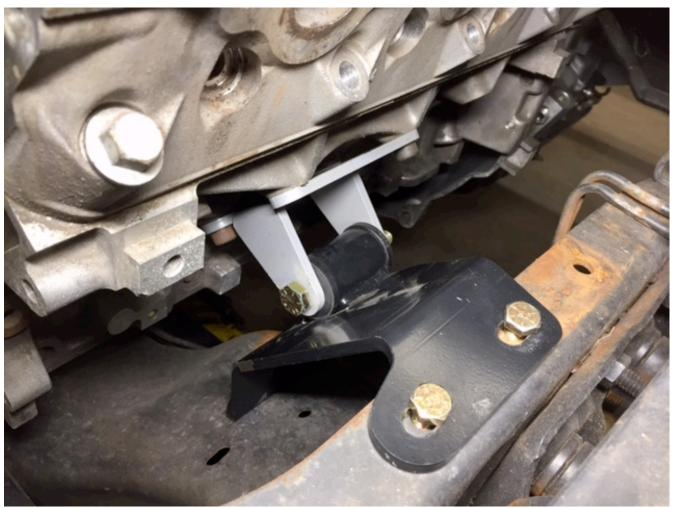
Step 3: Lower the engine/trans assembly into the chassis and align the frame brackets to the engine mounts holes and loosely install the  $\frac{1}{2}$ "-13 x 4" bolts, flat washers and nylon lock nuts.
