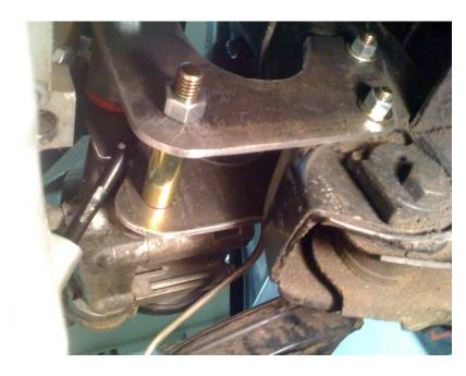
Here you can see how the dipstick tube runs through the notch in the mounting bracket. You may need to bend the dipstick tube slightly to get it to fit correctly.
