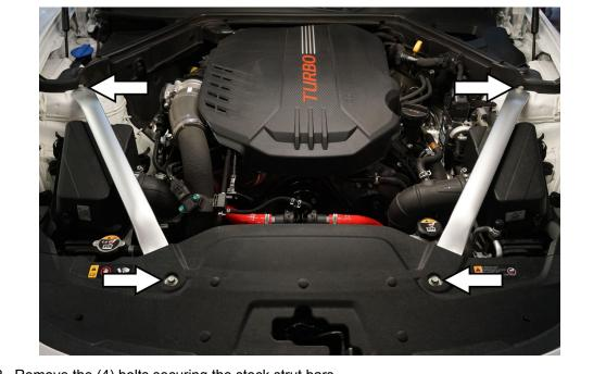
2. Remove the (4) bolts securing the stock strut bars.
