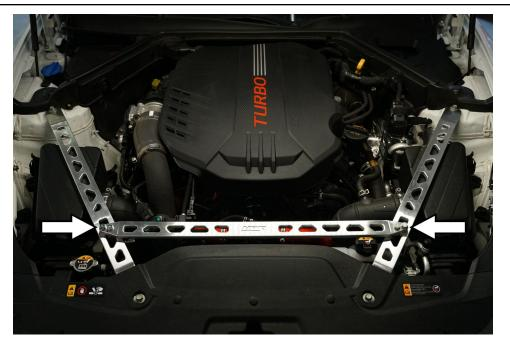
4. Install 42-105-C using the provided hardware (4) M8 bolts, (4) M8 split washers, and (4) M8 hex nuts as shown in the image above. Be sure to install the split washers and the M8 hex nuts on the underside of the strut bars with the bolt installed from the top down. Fasten all of the mounting hardware for the strut bars.
