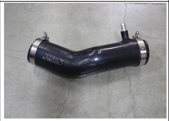
7. Install the T-bolt clamps onto the HPS silicone intake. Do not tighten the T-bolt clamps at this time.
