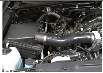
8. Insert the HPS intake onto the air box side first then onto the throttle body side. Reclip the upper part of the air box and adjust the HPS intake to the proper position.
