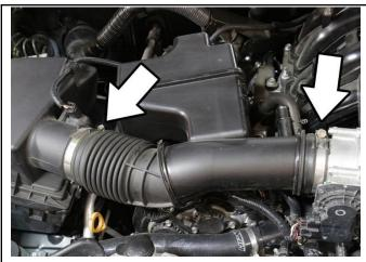
4. Loosen the hose clamp securing the throttle body and the air box. Locate the Mass Air Flow sensor harness clip on the resonator.
