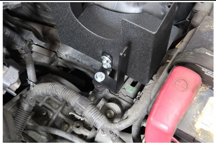
22. Loosely install the short ram intake bracket on top of the heat shield bracket using a washer and nut supplied in your hardware kit.
