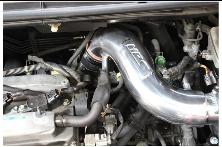
26. Reinstall the breather hose onto the intake pipe.
