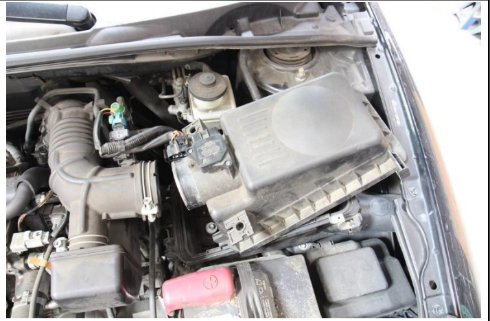
5. Remove the upper air box lid and the air filter from the vehicle.
