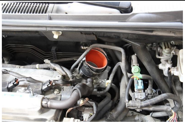
16. Install the reducer coupler along with the provided T-bolt clamps onto the throttle body.
