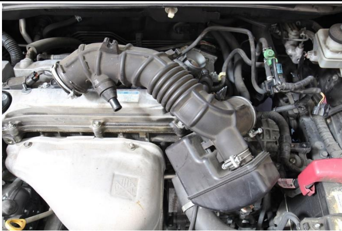
15. Remove the intake tube from the vehicle.
