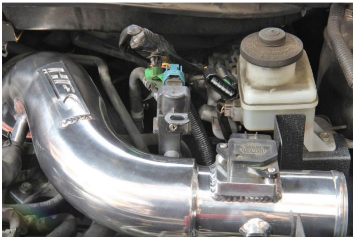
27. Reuse the factory screw to reinstall the EVAP sensor onto the sensor bracket along with the factory harness bracket.
