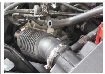
2. Remove the EVAP hose from the factory intake tube.
