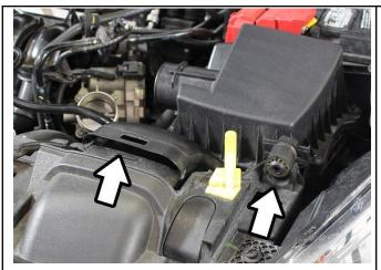
4. Pull off the air scoop and lift the air box from the rubber mount.
