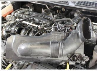
5. Carefully remove the air box assembly.
