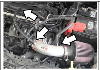
10. Install the breather hose that is provided in the hardware kit and re-connect the factory EVAP hose to the HPS intake. If vehicle is not equipped with an EVAP hose, install the provided vacuum cap onto the intake pipe.
