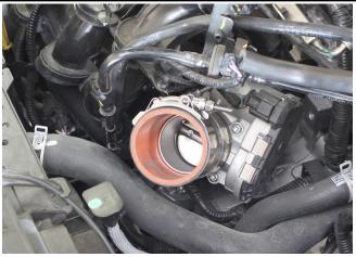
7. Slide the silicone coupler onto the throttle body, along with the two T-bolt clamps. Only tighten the clamp on the throttle body for now.
