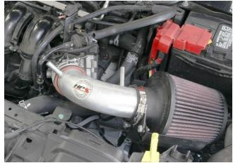
9. Press the HPS intake pipe into the coupler.
