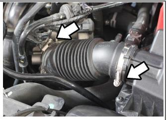
3. Loosen the clamps securing the throttle body and the air box and then remove the intake tube.
