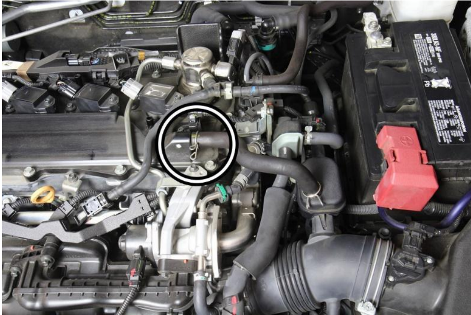
3. Loosen the hose clamp and remove the breather hose from the crankcase vent tube.
