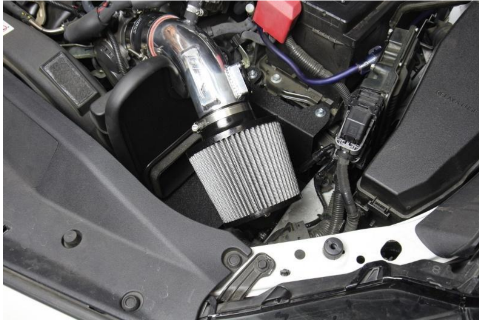
21. Install the HPS air filter onto the intake pipe.
