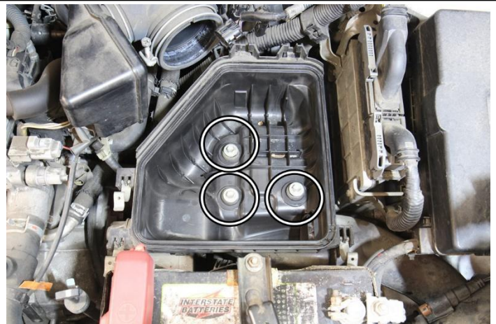
9. Remove the three 10mm bolts securing the lower air box.
