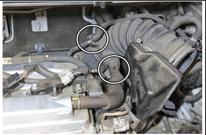
11. Disconnect the breather crank case hose from the intake tube and remove the EVAP hose from the intake tube.
