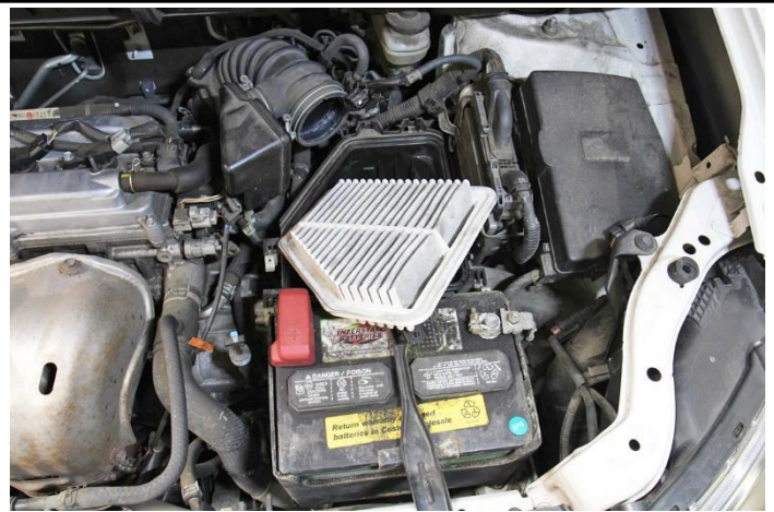
7. Remove the factory air filter from the vehicle.
