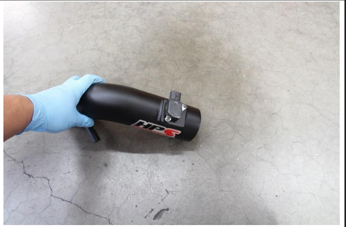
17. Remove the factory Mass air flow sensor from the air box and secure the sensor onto the HPS intake pipe using the two M4 Allen bolts provided in the hardware kit.
