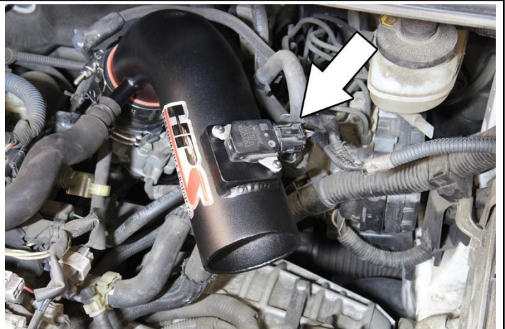
21. Reinsert the MAF sensor harness back into the MAF sensor.
