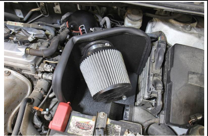
25. Insert the provided HPS performance air filter.
