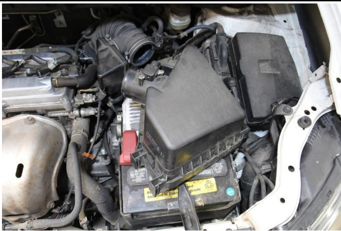
6. Disconnect the factory intake tube from the upper air box and remove it from the vehicle.
