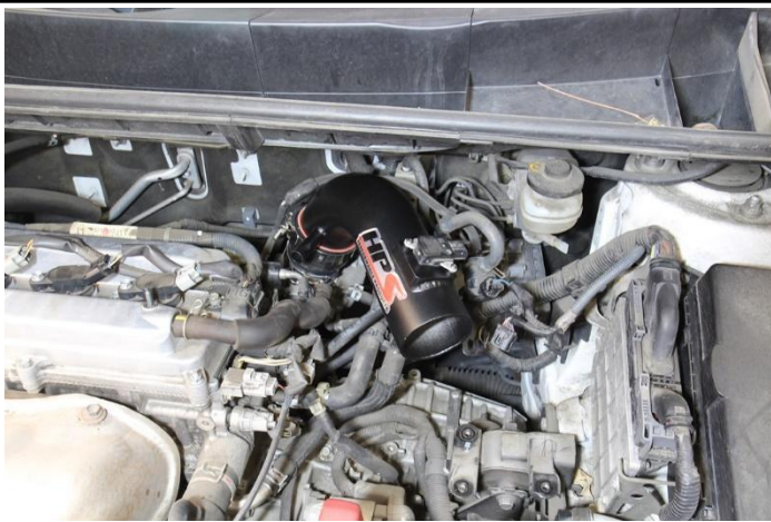
18. Insert the intake pipe into the throttle body coupler, but do not secure the intake pipe to the coupler yet.
