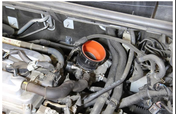
15. Install the reducer coupler along with the provided T-bolt clamps onto the throttle body.
