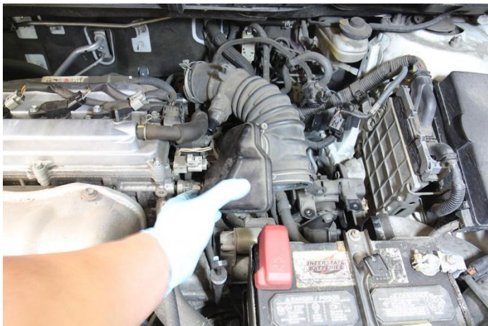
14. Remove the intake tube from the vehicle.
