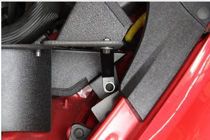
32. Install and secure the remaining heat shield bracket onto the heat shield. Secure the bracket with the provided M6x16 bolts, washers, and nuts.
