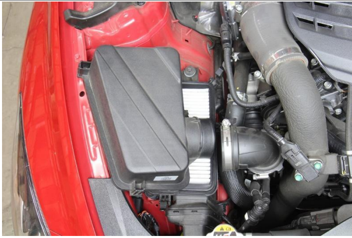
4. Separate the upper air box from the intake tube and remove the upper air box from the vehicle.
