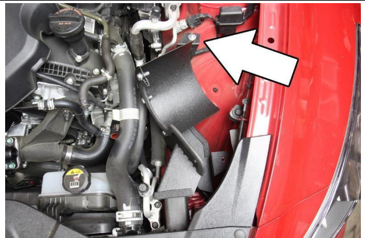
21. Insert the heat shield into the vehicle and secure the heatshield with a m6 nut and washer onto the vibration mount.
