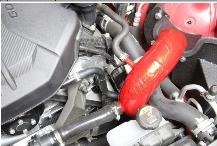
26. Insert the remaining breather hoses onto the intake barbs.
