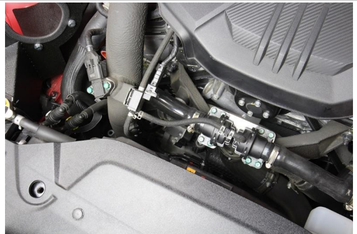
33. Insert and secure the remaining hose onto the BOV outlet with the provided hose clamp.
