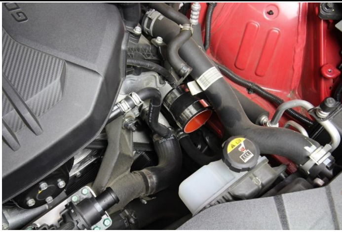
16. Install the coupler and the T-bolt clamps provided in the hardware kit onto the driver's side turbo inlet.
