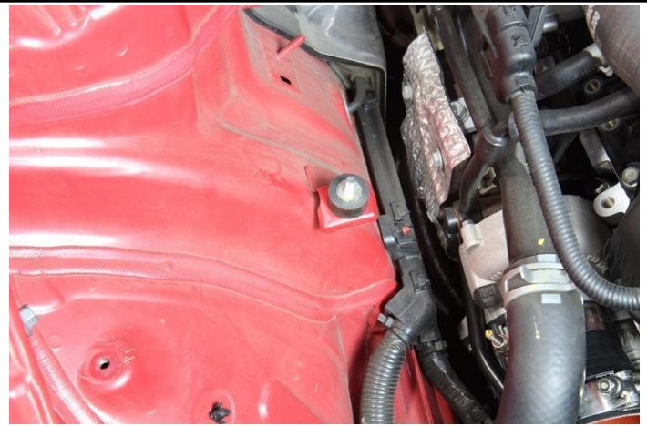
29. Install the 1/2" vibration mount onto the factory air box mount.
