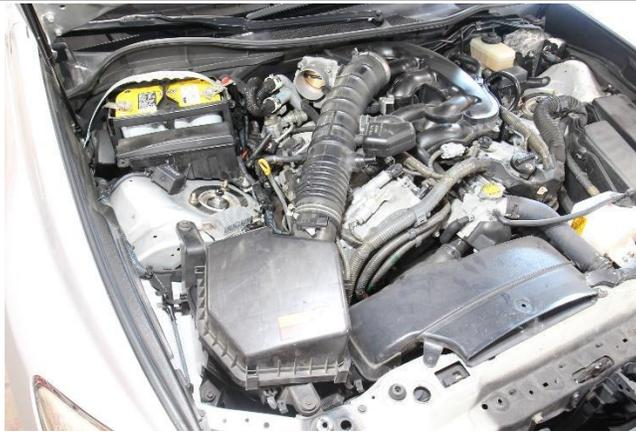
9. Remove the upper air box assembly along with the factory intake tube from the vehicle.
