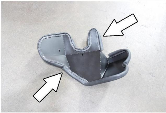
15. Install the provided bubble edge trim onto the HPS heat shield.
