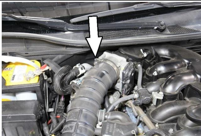
7. Loosen the hose clamp securing the intake tube from the throttle body.
