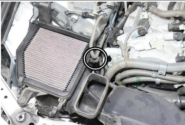
11. Disconnect the mass air flow sensor electrical harness from the lower air box assembly and remove the lower air box from the vehicle.
