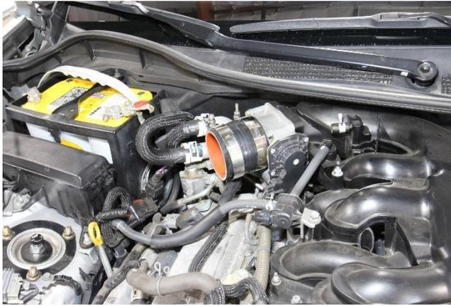
12. Insert the reducer coupler along with the provided T-bolt clamps onto the throttle body.
