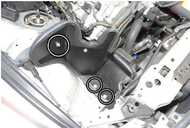
17. Insert and secure the heat shield onto the vibration mounts using the provided nuts and washers.
