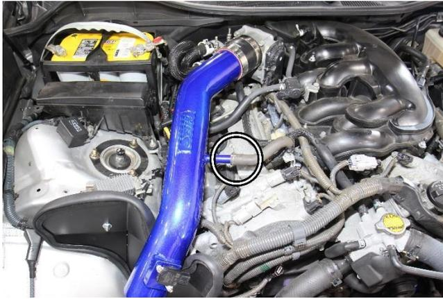
21. Reinstall the breather hose onto the intake pipe.
