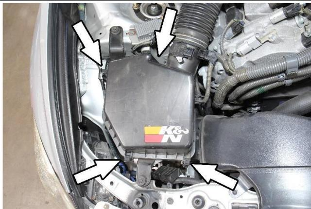
8. Unclip the four retaining clamps securing the upper air box assembly.
