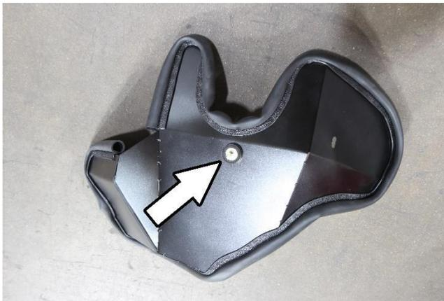
16. Install and secure the  $\frac{1}{2}$  vibration mount onto the heat shield shown above using a provided washer and nut.
