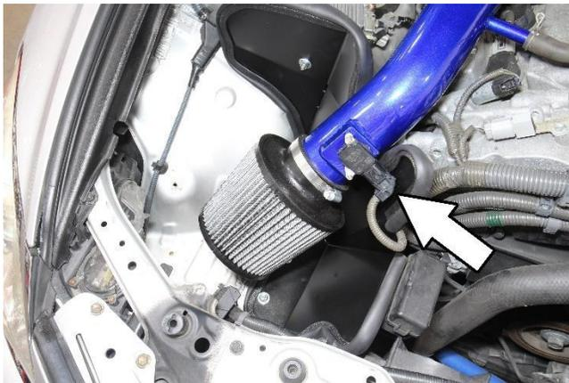
22. Reconnect the mass air flow sensor harness connector. Insert and secure the provided HPS performance air filter.
