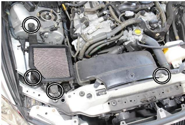
10. Remove 3x 10mm bolts from the lower air box assembly and 1x 10mm bolt from the air duct.
