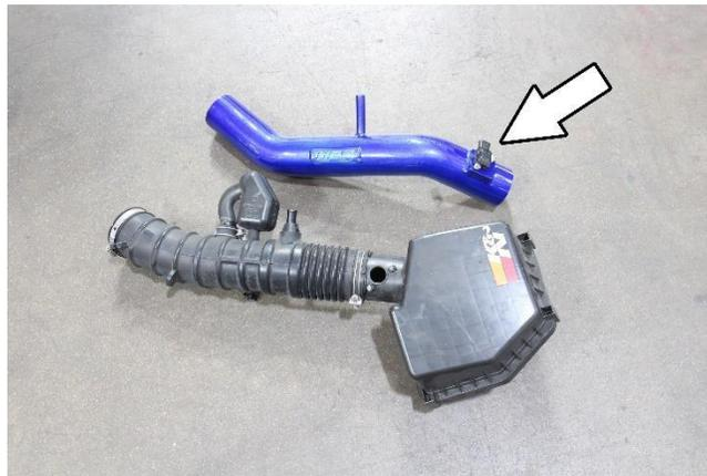
19. Remove and install the mass air flow sensor onto the HPS intake pipe using the provided M4 x 8mm allen bolts.
