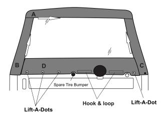
A) Start with the top zipper on the upper right side of the vehicle and zip in the rear window.
