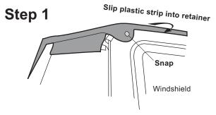
Lay the main skin out on the vehicle and insert the plastic strip into the channel over the front windshield. Now snap the front two snaps. Open the hook and loop flap on the sides over the front doors
