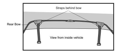
Make sure that the straps sewn into the rear of the top are behind the rear bow.
