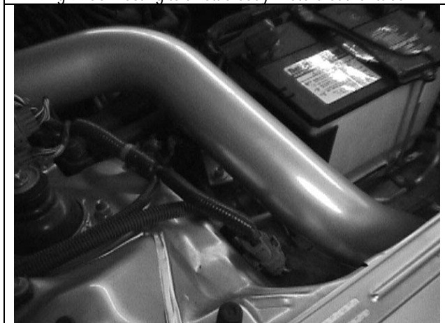
Fig 11: Air pipe installed. Note mounting bolt.
