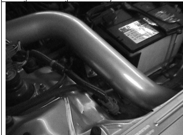
Fig 11: Air pipe installed. Note mounting bolt.
