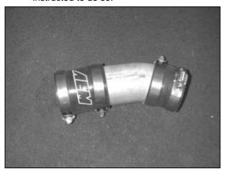
b. Install the 2.50" x 2.00" silicone hose on the shorter leg of the short AEM<sup>®</sup> intake pipe. Install one of the 2.50" x 3.00" silicone hoses on the longer leg of the same pipe. Loosely install two 2.50" hose clamps onto each silicone hose.
