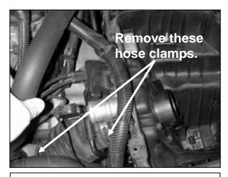
f. Loosen the two hose clamps on the rubber tube between the throttle body and intake manifold. Remove the rubber tube from the vehicle.
