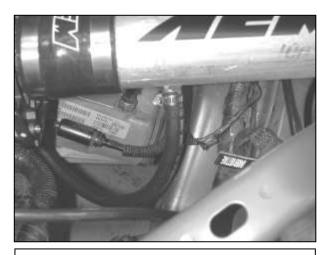
k. Connect the other end of the breather hose to the nipple on the AEM<sup>®</sup> intake pipe, secure in place with the remaining hose clamp. Route the hose carefully to prevent the hose from kinking.
