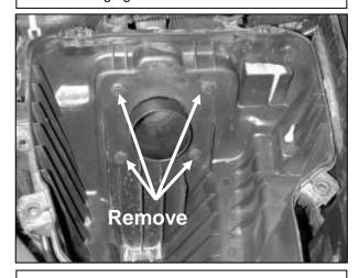
d. Remove the four screws that hold the throttle body to the lower airbox.
