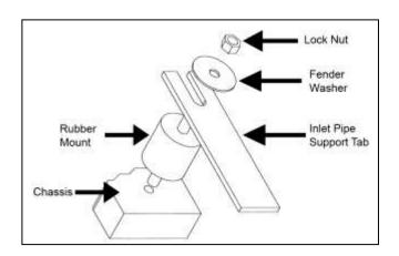
h. Proper installation of the rubber-mount assembly
