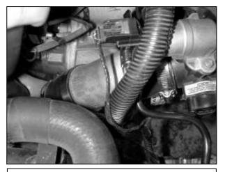
c. Install the short AEM<sup>®</sup> intake pipe between the intake manifold and the throttle body. The longer leg attaches to the intake manifold and the shorter leg attaches to the throttle body. Loosely tighten the hose clamps to hold the pipe in place, but do not fully tighten, as further adjustment may be needed.
