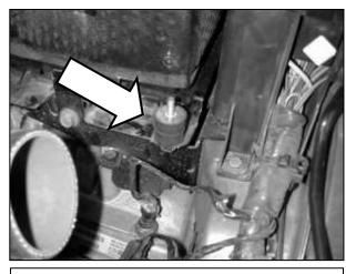
d. Remove the bolt from the right side of the battery tray and replace it with the supplied rubber mount.
