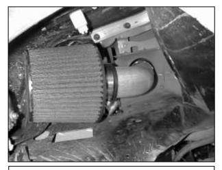
i. Install the AEM<sup>®</sup> air filter from the fender well of the vehicle. Position the air filter so that it is not in contact with any part of the vehicle, then tighten the hose clamp so it is secured to the intake pipe. Install the IAT sensor into the grommet installed in step 3f.
