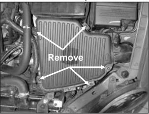
a. Loosen the five screws securing the stock airbox lid. Remove the airbox lid from the vehicle.
