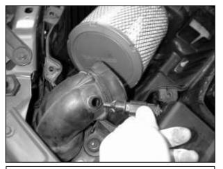
b. Remove the inlet air temperature (IAT) sensor. The metal band will need to be pried off with a flat-head screwdriver. Use care to avoid damaging the IAT sensor.
