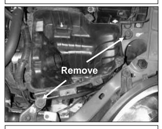
c. Remove the air filter element and the two lower airbox mounting bolts.
