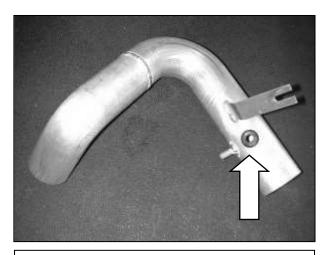
f. Install the supplied rubber grommet into the hole of the lower intake pipe.
