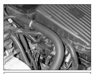
e. Remove the breather hose from the lower airbox. Remove the lower airbox from the vehicle.
