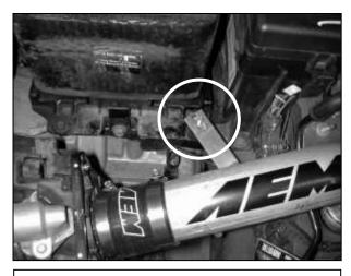
g. Install the lower intake pipe into the vehicle. Insert the intake pipe into the silicone hose on the throttle body. Loosely secure the hose clamps to secure the intake pipe in place. The bracket of the intake pipe should line up with the rubber mount installed in step 3d. Install the supplied washer and lock nut onto the rubber mount. Refer to the following diagram for proper installation of the assembly.
