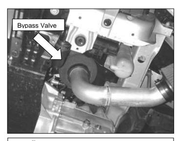
If AEM® Bypass Valve (part # 20-402S) is installed, install the bypass valve as shown in the figure above. The intake pipe will require modification so follow the instructions included with the AEM Bypass Valve accordingly.
