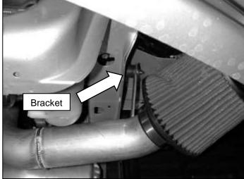
e. Secure the bracket to the rubber mount using the included washer and nylock nut and install the supplied air filter.
