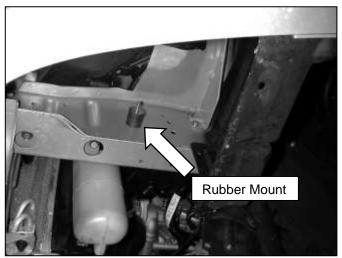
c. Install the AEM® rubber mount into the treaded hole in the outer frame rail, as shown.
