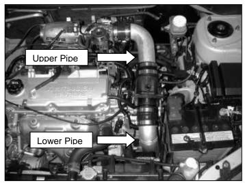
d. Install the upper intake pipe, MAF assembly, lower intake pipe and supplied couplers and hose clamps. Install the cam cover breather hose, as shown. Use the included clamp to secure the breather hose to the intake pipe.
