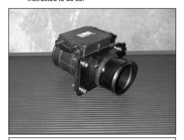
b. Using the included socket head bolts and nylock nuts, bolt the supplied MAF adaptor to the factory MAF sensor, as shown.
