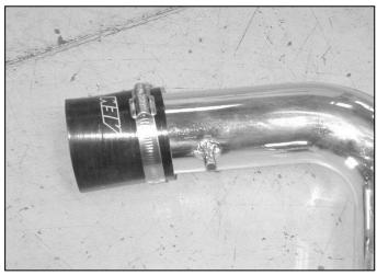
c. Check to see that the inside of the upper intake pipe are clean and free from any foreign objects and/or obstructions. Install the 2.75" silicone coupler over the throttle body end of the pipe using the 2.75" hose clamp.
