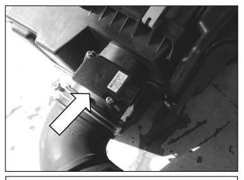
i. Remove the two bolts securing the MAF sensor to the air filter housing and remove the MAF sensor. **NOTE: Be careful not to damage the sensor.**
