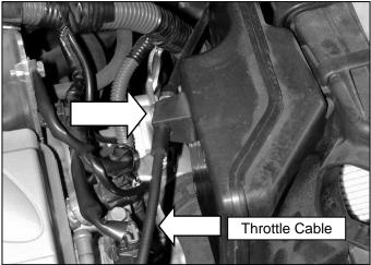
d. Unclip the throttle cable from the side of the air filter housing.
