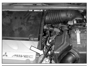
c. Remove the breather hose from the valve cover by pulling it off.
