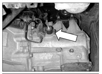
b. Remove the driver's side bolt securing the slave cylinder bracket to the transmission. Thread in the supplied rubber mount as shown.
