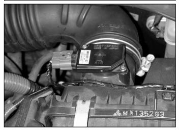
g. Unplug the MAF sensor from the engine harness.
