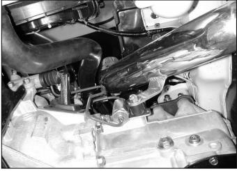
I. Ensure the air filter is not touching any part of the vehicle. Position the AEM® intake for best fitment. Be sure that the pipe or any other component is not in contact with any part of the vehicle. Tighten the hose clamps at the throttle body and silicone coupling. Tighten the nut on the mounting bracket. Re-adjust the pipe if necessary.
