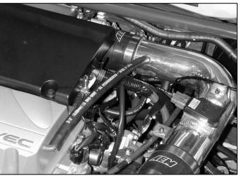
j. Plug in the MAF sensor and secure the wiring harness using the supplied tree mount zip tie. Install the supplied 3/8" breather hose onto both the valve cover nipple and the pipe nipple. Use the supplied 3/4" hose clamps to secure. Trim for proper fitment. Secure the throttle cable using the supplied tree mount zip tie. Trim the excess plastic zip strap.
