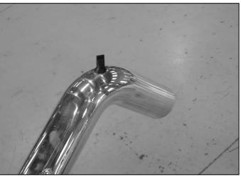
f. Install the supplied duck-bill drain into the  $\frac{1}{2}$ " hole on the lower intake pipe. This drain prevents water from building up in the bottom of the intake pipe due to the angle in which the filter is placed.
