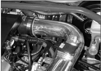
d. Slide coupler attached to the upper intake pipe over the throttle body using the supplied 2.75" hose clamp.
