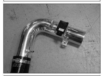
d. Install the previously removed MAF sensor into the upper intake pipe using the two supplied allen bolts.
