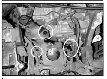
k. Remove the three bolts securing the air box bracket to the car. Remove the bracket.
