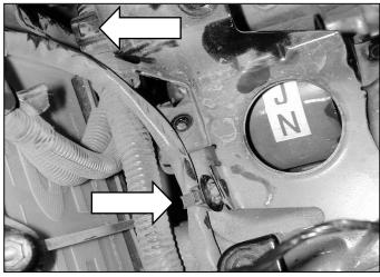
j. Unclip the wiring harness from the air box bracket behind the batery.
