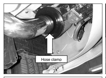
i. Install the AEM<sup>®</sup> air filter onto the end of the intake pipe. Push the air filter over the intake pipe until the stop in the air filter is reached. Then install one hose clamp to secure the air filter onto the intake pipe. Once proper fitment is achieved, tighten the hose clamp.
