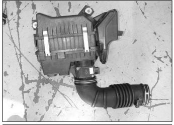
h. Remove the two bolts securing the stock air filter housing to the engine bay. Remove the air filter housing and the inlet tube.
