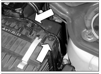
e. Unclip the Mass Air Flow (MAF) sesnor wiring harness from the air filter housing. These clips can be removed undamaged from the harness using a small flat head screwdriver.
