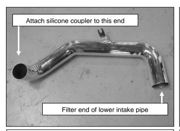
e. Ensure that the inside of the lower intake pipe and air filter are clean and free from any foreign objects and/or obstructions. Install the 2.75" silicone coupler over the end of the pipe using the 2.75" hose clamp.
