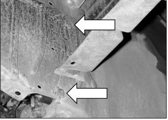
I. Raise the front of the vehicle with a jack. Refer to your owner's manual for proper jack and jack stand placement to properly support vehicle. Support your vehicle using properly rated jack stands before wheel removal or while working under the vehicle.
