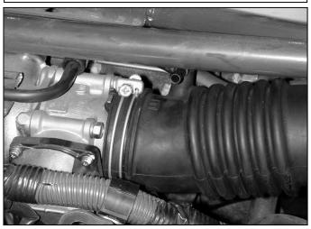
f. Unscrew the inlet tube from the throttle body and pull the inlet tube off the throttle body.
