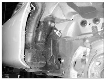
k. Remove the left fender liner to expose the lower air box / washer bottle assembly.
