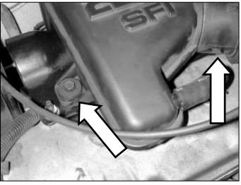
d. Remove bolt. Release the breather hose from the valve cover.
