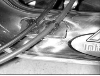
k. Secure the throttle/cc cable(s) to the upper pipe with the zip tie(s) installed earlier. Cut off excess material.
