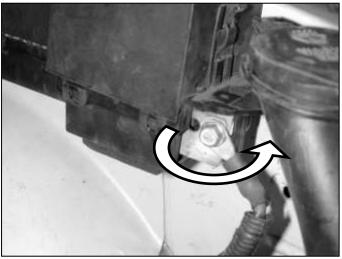
r. Loosen the positive lead on the fuse block.  $\mbox{\bf Rotate\ it}$  as shown. Tighten the lead.
