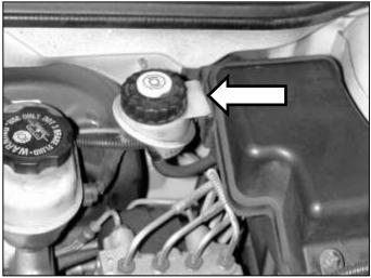
j. If equipped with a manual transmission, remove the clutch fluid reservoir from the air box. Secure it to the firewall with AEM® part # 20-445. Remove the air box from the vehicle.
