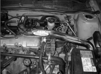
AEM® intake system installed
