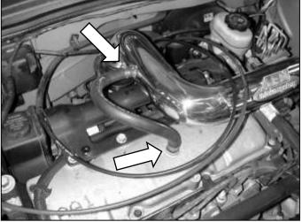
m. Install the supplied breather hose between the valve cover and intake pipe. Secure it with the supplied hose clamps.
