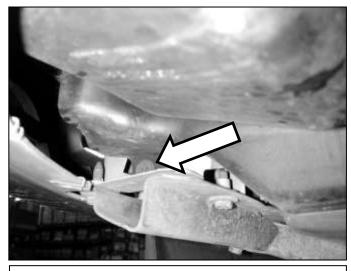
o. Remove the lower bolt near the front of the washer bottle.
