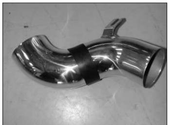
d. Mark the pipe approximately  $\frac{1}{2}$ " above and below the hole in the fender. Remove the pipe and apply the adhesive neoprene material as shown. Reinstall the intake pipe as previously directed.
