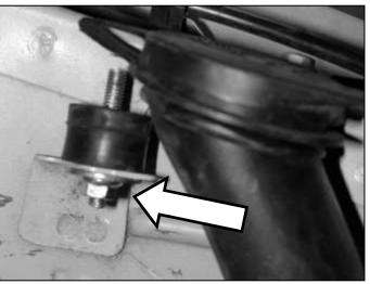
g. Attach the rubber mount to the tab near the washer bottle filler neck using the supplied washer and lock nut.
