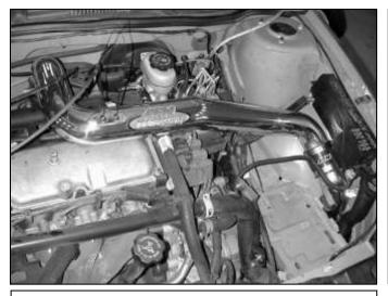
j. Place the upper intake pipe in the engine bay as shown.
