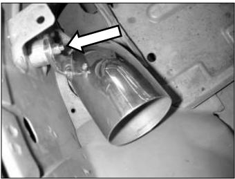
c. Install spacer as shown. Install the lower pipe in the engine bay. Center the pipe in the hole in the fender and tighten the nut on the spacer.
