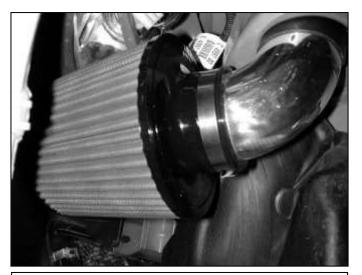
p. Install the air filter onto the end of the intake pipe.
