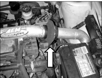
AEM® bypass valve installed.
