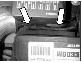
o. Reinstall the battery. Confirm that the positive lead from the fuse box is on top of the intake pipe and is not pinched between the battery and the intake pipe.
