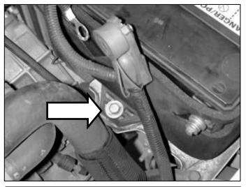
g. Remove the battery by first releasing the tie down bolt.
