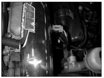
I. Insert the IAT sensor through the grommet in the upper pipe. Do not push the grommet into the pipe.
