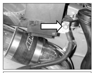
n. Check the fitment of the pipes and tighten all hose clamps. Secure the fuse block to the rubber mount with the supplied lock nut and washer.
