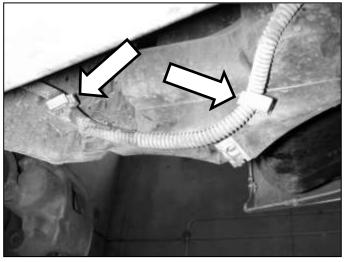
I. Release the two wire clamps on the back of the washer fluid bottle.
