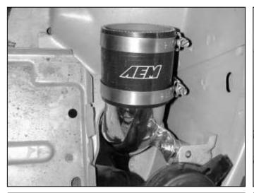
f. Install the supplied silicone hose as shown. Orient the hose clamp screws away from the battery tray as shown.
