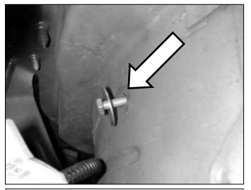
b. Install supplied bolt and washer through fender as shown. This picture was taken from inside the fender well.
