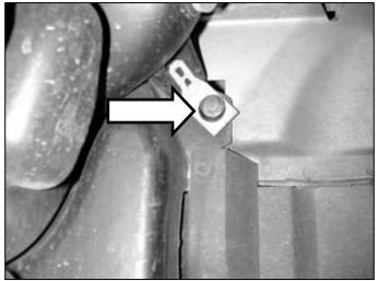
n. Remove the bolt that secures the washer bottle to the fender.
