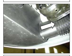
h. Pull the air snorkel from the splash shield and remove the splash shield.
