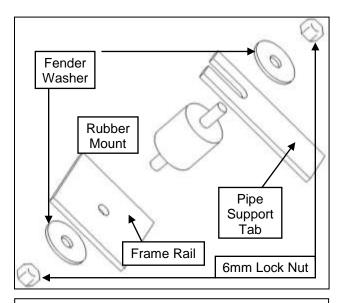
h. Proper installation of the rubber mount assembly.
