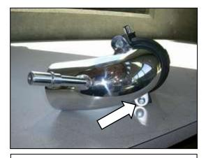
c. Secure the upper inlet pipe to MAF housing with the supplied bolts.
