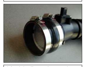
d. Attach the silicone reducer onto the MAF sensor housing.
