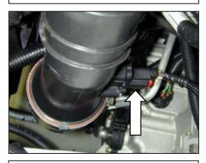
f. Connect the MAF sensor wire harness to the MAF sensor.
