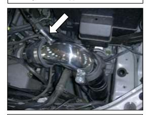
e. Install the upper intake pipe onto the throttle body. Attach the breather hose to the intake pipe's nipple.
