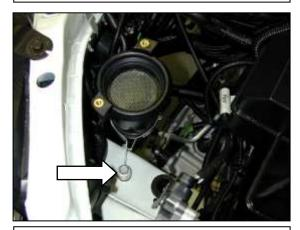
d. Remove the upper airbox and the bolt in the frame rail. Release the metal clamp from the Mass Air Flow (MAF) sensor housing.
