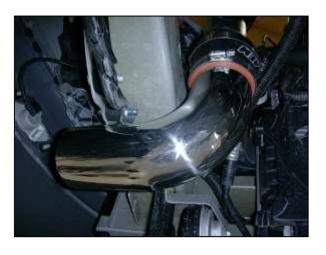
i. Install the lower intake pipe into the lower coupler of the MAF sensor housing. Align the intake pipe's bracket with the rubber mount secured to the frame rail.
