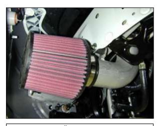
j. Secure the AEM<sup>®</sup> air filter onto the end of the lower intake pipe with the provided hose clamp.
