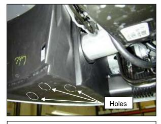
k. Reinstall the splash shield. Drill ½" holes in the bottom of the splash shield to facilitate water drainage.
