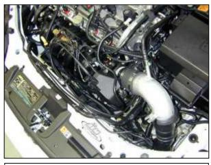
AEM® intake system installed
