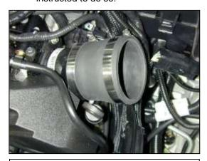
b. Install the rubber reducer with two hose clamps onto the throttle body.
