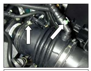
Release the fitting on the inlet pipe nipple and loosen the hose clamp at the throttle body.
