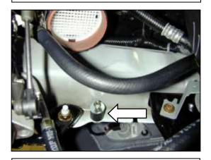
g. Install the rubber mount into the frame rail with a supplied washer and lock nut.
