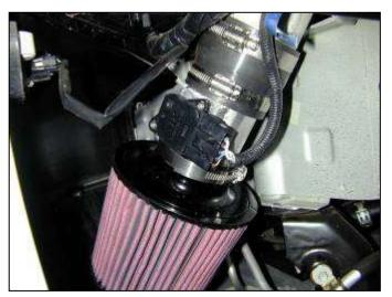
I. Attach the air filter apparatus as shown. Route the stock air flow sensor wiring harness through the hole in the fender and plug it into the sensor as shown. Again check the position of the air flow meter and confirm that is positioned as shown above.
