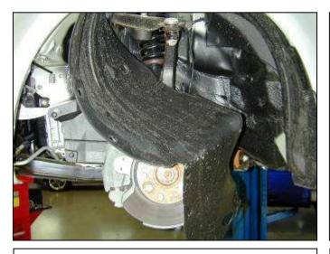
k. Place the partially removed fender liner as shown.
