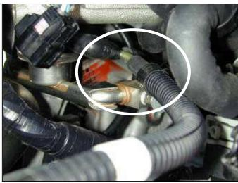
c. Follow the vacuum hose from the air box up to the plastic vacuum fitting under the throttle body. Carefully pull the vacuum hose off of the fitting. Be careful not to break it. Remove hose form vehicle.
