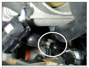
d. Install supplied vacuum cap onto the open port on the vacuum fitting.
