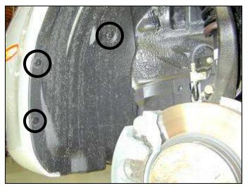
i. Release plastic clips inside the fender.
