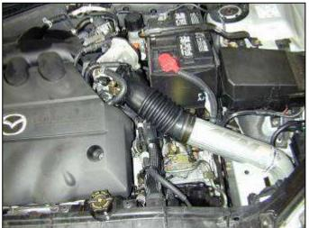
AEM® intake system installed
