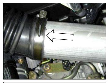
j. Secure the upper end of the pipe utilizing the stock inlet hose and clamp. A small amount of WD-40 on the end of the pipe may ease installation.
