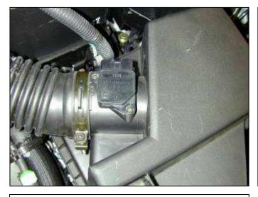
c. Release all clips and remove upper air box from vehicle.
