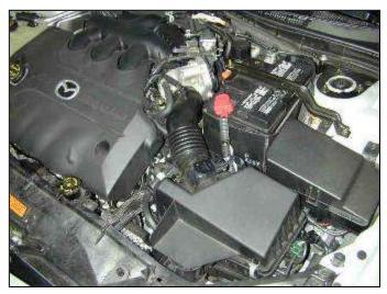
a. Stock air box system installed.
