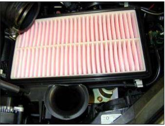
d. Remove the air filter from lower air box.
