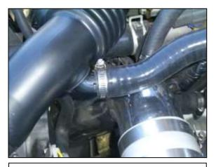
t. Attach the connector end to the BOV hose return side. Secure with hose clamp.
