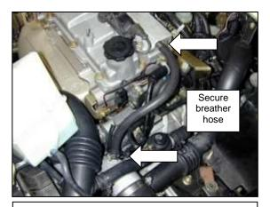
q. Attach crank case breather hose and secure with hose clamps.
