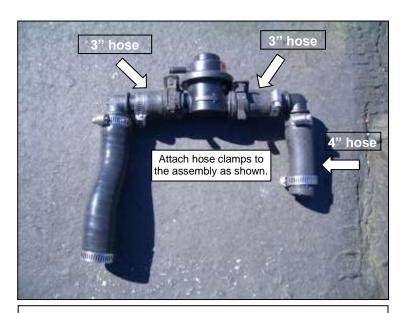
r. Assemble BOV return hose like above. The stock hose attaches on the same side as the nipple on the BOV. Attach the 3" hoses to the BOV. The stock spring clamps are used to at the BOV. Insert 90 degree elbows into each end of the 3" hoses. Secure with hose clamps. The stock hose attaches to the same side as the nipple on the BOV. On the opposite side attach the 4" hose and secure with hose clamps.
