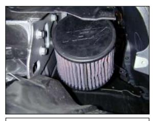
I. Attach the AEM air filter element onto the end of the inlet pipe. Make sure the air filter clears the body and splashguard. Secure the air filter's hose clamp.
