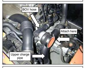
d. Attach coupler and hose clamps to the intake pipe. Make sure the pipe clears the upper charge pipe and BOV hose.
