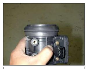
f. Remove the rubber gasket. This piece will not be reused.
