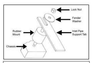
Proper rubber mount assembly installation.
