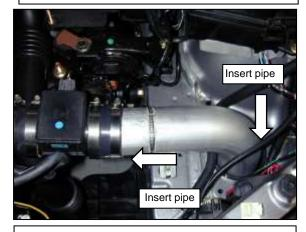
k. Insert the lower intake pipe into the lower cavity. Then insert the pipe into the coupler with the MAF Sensor. Align with the rubber mount.
