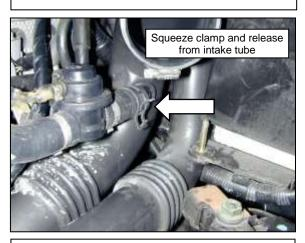
h. Squeeze clamp and release blow off valve hose from the specified intake tube.
