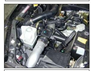
x. Reinsert the coolant reservoir on the new bracket.
