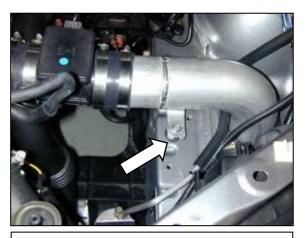
m. Secure inlet pipe at the bracket on the rubber mount.
