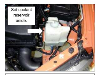
d. Remove the radiator fluid overflow bottle and set aside in the engine bay. Do not disconnect the any of the coolant lines. There should be plenty of slack in the hose.
