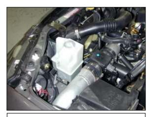
p. Attach the coolant overflow reservoir to the new bracket.
