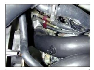
j. Loosen hose clamp and remove intake tubing from the turbo inlet.
