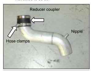
b. Assemble the turbo intake pipe as shown.
