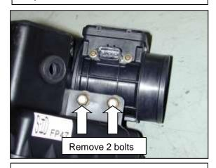
e. Remove the 2 bolts holding the MAF sensor. Carefully remove the MAF sensor from the air box.
