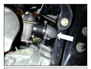
c. Attach the reducer coupler, hose clamps and inlet pipe to the turbo inlet. Make sure to clear the fan shroud. Use the 2.5-2.75" coupler.
