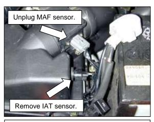
b. Unplug the MAF sensor and remove the IAT sensor from the air box.
