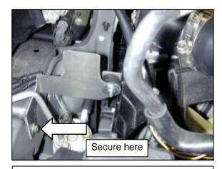
o. Secure the coolant reservoir-mounting bracket to the rubber mount and also to the frame.
