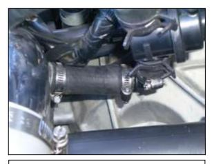
s. Attach the 4" end to the turbo intake pipe and secure with provided hose clamp.
