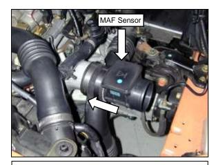
g. Insert the MAF sensor into the coupler. Make sure the MAF sensor is pointing up and the plug for the harness is pointing towards the firewall.
