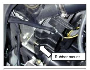
n. Secure rubber mount to the radiator tab support.
