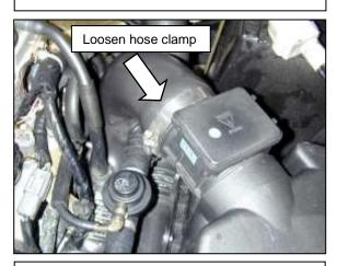
g. Loosen and remove hose clamp. Remove the air box assembly.
