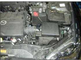
a. Factory air box system installed.
