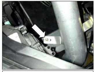
k. Secure the pipe bracket to the rubber mount using a flat washer and 8mm nut.
