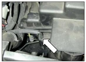
d. NOTE: 2007-2008 model year vehicles do not have vacuum solenoid. Proceed to step e. Pull the vacuum hose off of the air box nipple.
