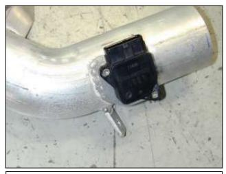
c. Install the previously removed MAF sensor into the inlet pipe using the two supplied bolts.
