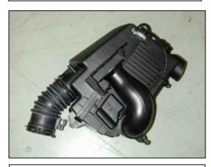
g. Gently pull the air filter housing up and out of the engine bay.
