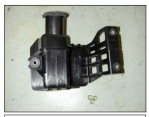
m. Remove the lower resonator.
