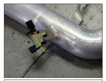
e. NOTE: 2007-2008 models do not have vacuum solenoid. Proceed to step 3g. Attach the vacuum solenoid to the intake pipe using the supplied flat washer and the previously removed nut.
