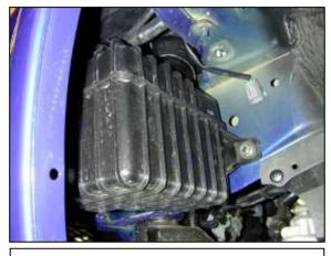
I. Remove the three nuts that secure the lower resonator to the chassis.
