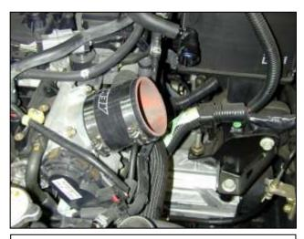
g. Attach the silicone coupler to the throttle body using the supplied #44 hose clamp.
