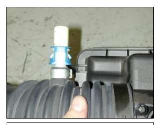
o. Carefully remove the blue plastic clip from the stock intake hose nipple. This can be done by gently prying the two tabs up and over the retaining ring with a small object such as a paperclip
