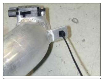
d. Install the supplied tree mount zip-tie into the bracket with the  $\frac{1}{4}$ " hole on the pipe.
