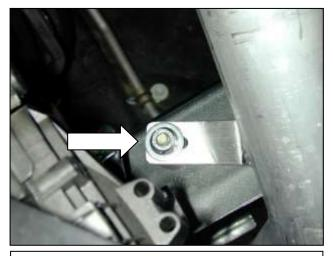
i. Check that the inside of the AEM<sup>®</sup> upper intake pipe is free and clear of any debris. Slide the pipe into the hole where the lower resonator was located and align the mounting bracket with the rubber mount previously installed in step 3h.
