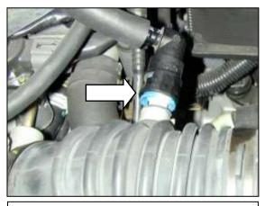
e. Remove the plastic crankcase breather hose by pinching the blue connector and pulling on the hose.
