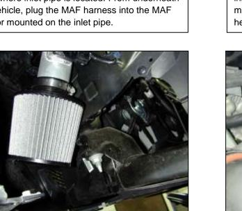
n. Install the AEM<sup>®</sup> air filter on to the end of the inlet tube. Push the air filter over the inlet pipe until the stop in the air filter is reached. Install and fully tighten one #48 hose clamp to secure.
