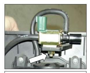
p. NOTE: 2007-2008 models do not have vacuum solenoid. Proceed to step q. Remove all the vacuum lines connected to the vacuum solonoid on the air filter housing. Remove the vacuum solenoid from the air filter housing by removing the nut securing it.
