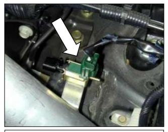
p. NOTE: 2007-2008 models do not have vacuum solenoid. Proceed to step 4. Plug in the vacuum solenoid harness.
