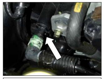
f. Cover the open nipple exposed during step 2q with the supplied vacuum cap.
