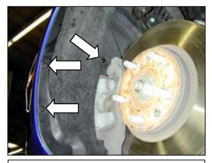
i. Raise the front of the vehicle with a jack. Refer to your owner's manual for proper jack and jack stand placement to properly support vehicle. Support your vehicle using properly rated jack stands before wheel removal or while working under the vehicle. **NEVER WORK UNDER A VEHICLE WITHOUT USING JACK STANDS.** Remove the front driver side wheel. Release the three plastic rivets securing the fender liner.
