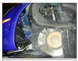
k. Move the fender liner so the lower resonator becomes accessible.
