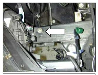
h. Install the supplied rubber mount into the front threaded hole where the air filter housing mount was secured.
