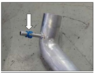
b. Install the plastic breather hose clip onto the  $\mathsf{AEM}^{^{\textcircled{B}}}$  intake pipe.
