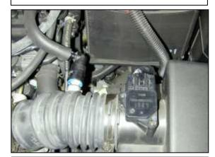
c. Unplug the MAF sensor from the wiring harness. Unclip the wiring harness from the back of the air filter housing.
