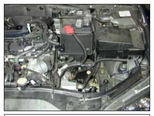
r. Factory air box system removed
