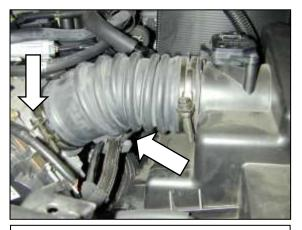
f. Loosen the hose clamp at the throttle body. Unhook the hoses from the bottom of the inlet hose. Pull the inlet hose off of the throttle body.
