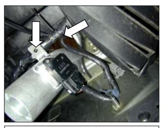
m. Secure the headlight wiring harness to the inlet pipe using the previously installed tree mount zip-tie. Secure the MAF harness to the headlight harness with the other zip-tie.
