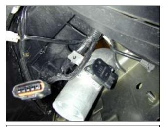
I. Route the MAF sensor harness through the hole where inlet pipe is located. From underneath the vehicle, plug the MAF harness into the MAF sensor mounted on the inlet pipe.
