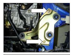
h. Remove the air filter housing mount by removing the two bolts securing it to the chassis.
