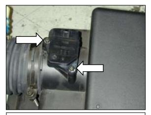
n. Remove the stock MAF sensor from the air filter housing. Be careful not to damage the MAF sensor.
