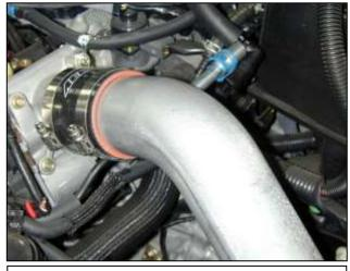
j. Slide the pipe into the silicone coupler on the throttle body and secure using a #44 hose clamp.
