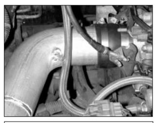
f. Install the inlet pipe into the coupler as shown. Secure in place using the #48 hose clamp. Install the supplied breather hose onto the valve cover breather and the nipple of the intake pipe. Secure in place with the supplied hose clamps.
