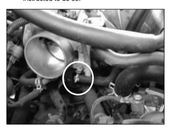
b. CAUTION: Ensure the engine is completely cool before removing the coolant hose, or hot coolant will escape from the cooling system and cause injury or damage. Be sure to capture any lost coolant in a clean container. Disconnect the water bypass hose from the bottom of the throttle body. Install the supplied 5/16" hose and secure with a 3/4" hose clamp.
