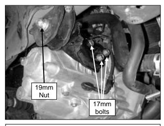
a. Using a 19mm socket, remove the engine mount nut. Loosen the three bolts with a 17mm wrench and remove the mount.
