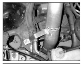
g. Align the aluminum mounting tab with the rubber mount installed earlier in step #4e. Use the supplied nylock nut and washer to secure the bracket in place. Refer to the diagram below on the next page for proper rubber mount installation.
