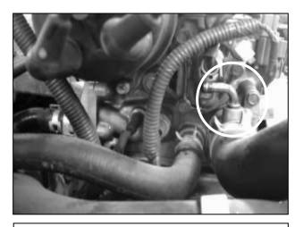
c. Remove the other end of the water bypass hose from the fitting on the engine. Install the opposite end of the 5/16" hose onto this fitting and secure in place with a 3/4" hose clamp.
