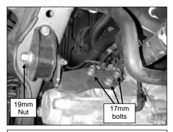
d. Using the supplied bolts and washers, install the AEM® engine mount on the transmission, torque the bolts to 61ft-lb. Then replace the factory washers and nut on the mounting stud.
