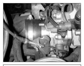
d. Install the supplied reducer coupler onto the throttle body and secure using the #44 hose clamp.
