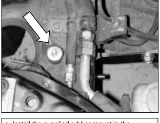
e. Install the supplied rubber mount in the threaded hole in the stock fender well as shown.
