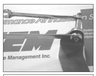
c. Install the factory mounting stud removed in step #3b through the supplied engine mount bracket. Secure in place with the provided nylock nut and washer.
