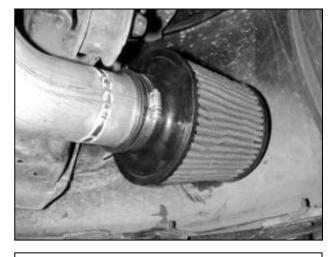
Proper installation of the rubber mount assembly.
