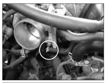
b. CAUTION: Ensure the engine is completely cool before removing the coolant hose, or hot coolant will escape from the cooling system and cause injury or damage. Be sure to capture any lost coolant in a clean container.
