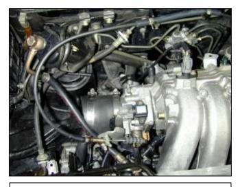
d. Attach the reducer coupler. Secure the 2.75" end onto the throttle body with provided hose clamps.
