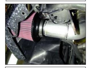
q. Attach the air filter to the lower inlet pipe, ensuring proper fitment and sufficient clearance. Secure the air filter to the inlet pipe with the provided hose clamp.
