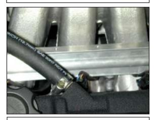
n. Attach the breather hose to the valve cover and secure with the provided hose clamp.
