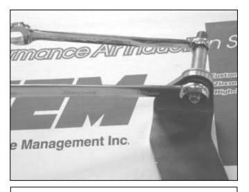
h. Install the factory mounting stud removed in step #3g through the supplied engine mount bracket. Secure in place with the provided washer and Nylock nut.
