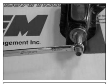
g. Using a 14mm wrench, remove the mounting stud from the factory engine mount assembly. It may be necessary hold the bracket in a vice to do this.
