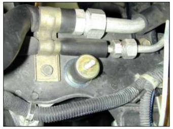
k. Insert the rubber mount on top of the ¼" washer and secure in place.
