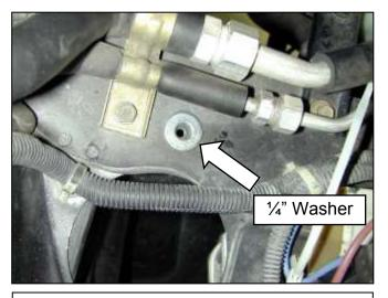
j. Locate the mounting hole next to the A/C line behind the passenger headlight. Place the ½" spacer over the hole as shown. It will sit between the rubber mount and the vehicle body.
