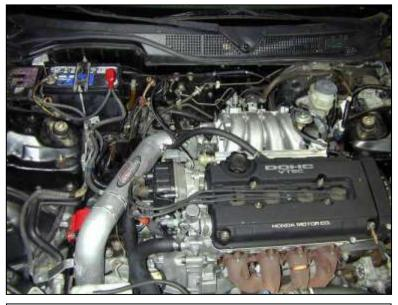
AEM® intake system installed
